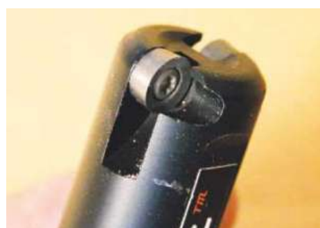
▲ The cutters are made from solid tungsten carbide for durability
